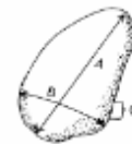
A = LONGEST AXIS (LENGTH) B = INTERMEDIATE AXIS (WIDTH) C = SHORTEST AXIS (THICKNESS)
